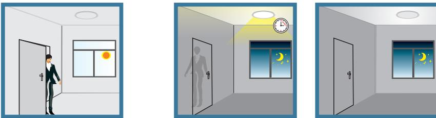
If with sufficient ambient light, the lamp turns off at once, even with motion trigger.
